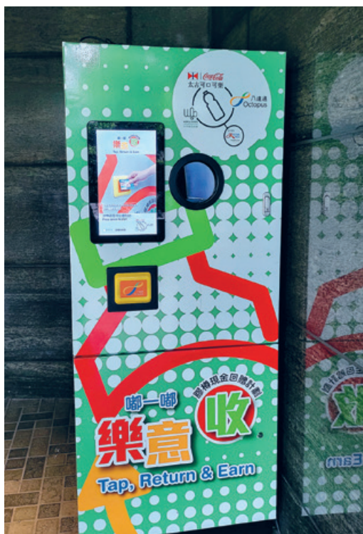
Left: A Reverse Vending Machine at Festival Walk that collects used beverage bottles for recycling.
